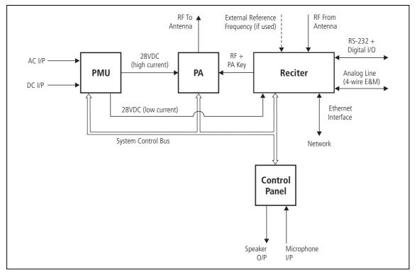
The reciter carries out signal processing and has overall control of the base station. It comprises an RF, a digital, and a network board, as shown in Figure 1.3.
