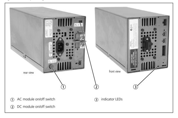
Figure 4.5 Operating controls on the PMU
