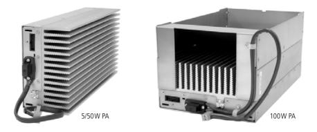
All three models are designed to operate on the 28 VDC output provided by the TB9100 power management unit. In addition, variants of the 5 W and 50 W models are available for DC-only operation. These two 12 V PAs are fitted with an internal boost regulator board, which converts the 12 V nominal DC input to a 28 VDC output to power the PA circuit boards. The boost regulator board also provides a 12 VDC output to power the reciter.
