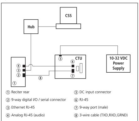
Figure 3.3 TB9100 to CTU connections
