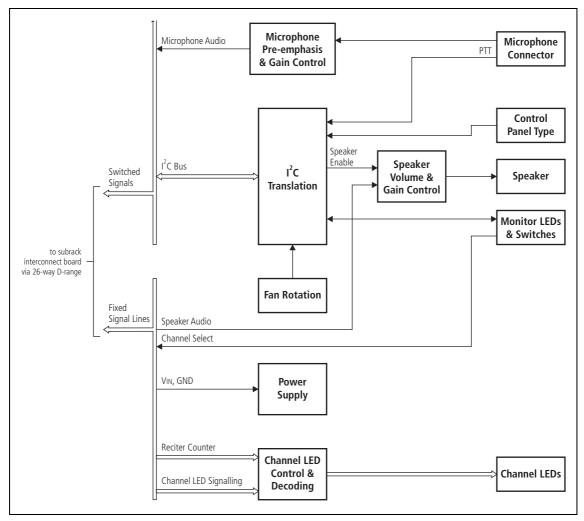
**Audio Circuitry** The volume of the speaker is controlled by the volume control knob. In addition, the control panel performs gain control so that, with an input of 167 mV pp, the power output into a 16 $\Omega$  speaker is  $\geq 0.5$  W at the maximum position of the knob, and 0 W at the minimum position of the knob. Speaker audio is from the currently selected reciter only. An LED indicates when the speaker is on.
