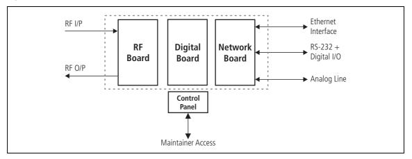
The RF board contains the receiver and exciter circuitry.
