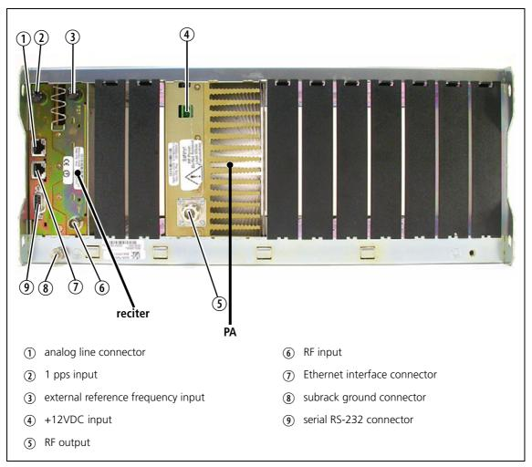
Figure 3.9 5W or 50W 12V DC PA-only base station inputs and outputs
