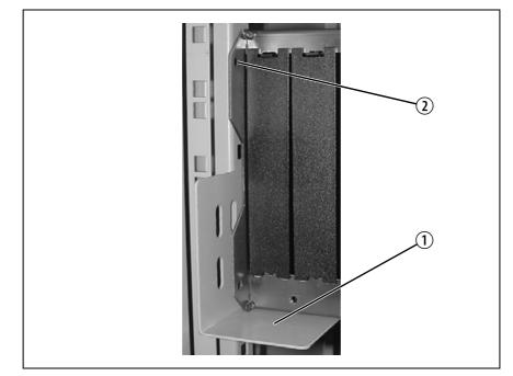
Figure 3.6 Optional slide mounting rail - rear view
