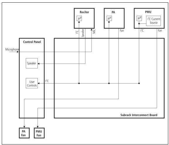
Figure 1.5 Intermodule communication paths
