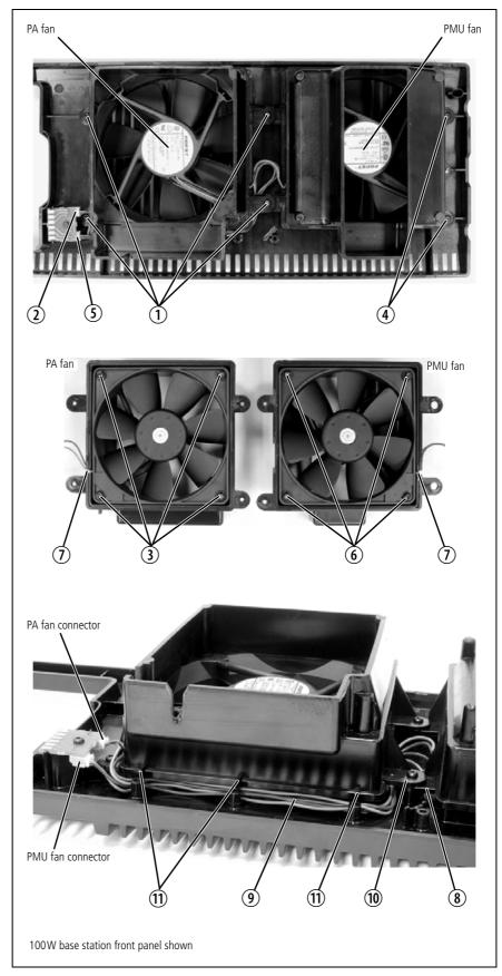
Figure 7.1 Replacing the front panel fans
