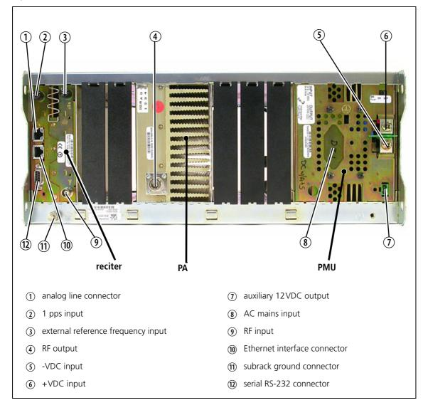
The connections at the rear of a 12V DC PA-only base station with a 5 W or 50 W PA are identified in Figure 3.9.
