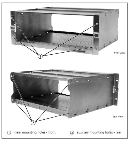
Figure 3.4 Subrack mounting points
