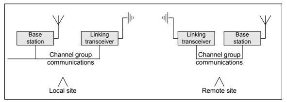
A TB9100 must be appropriately configured using the CSS before it can function as a linking transceiver. As voting information cannot be carried over the RF link, signals that the linking transceiver provides to its channel group must be assigned a source type and given a fixed impairment value. For details, see the TaitNet P5 System Manual and the CSS manual or online Help.
