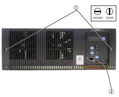
2. While supporting the left end of the front panel, place your fingers in the recess provided on the left side of the control panel opening ② and pull the right end of the front panel away from the subrack. You will need to overcome the resistance of the spring clip securing the front panel to the control panel.
