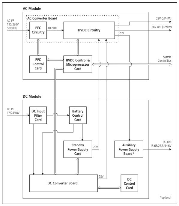
Standby Power Supply The standby power supply card plugs into the DC converter board and provides power to the reciter output. This allows the main DC unit to be switched off to reduce current consumption in low-power situations, e.g. when the PA is not transmitting.
