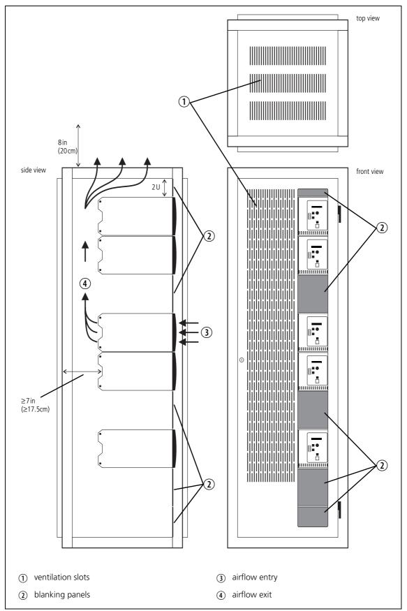
Figure 3.1 Typical cabinet ventilation requirements
