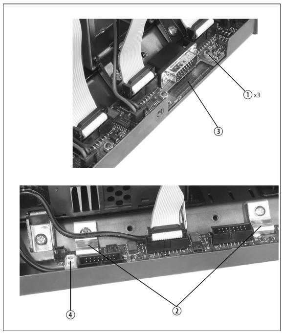
Figure 7.2 Replacing the subrack interconnect board
